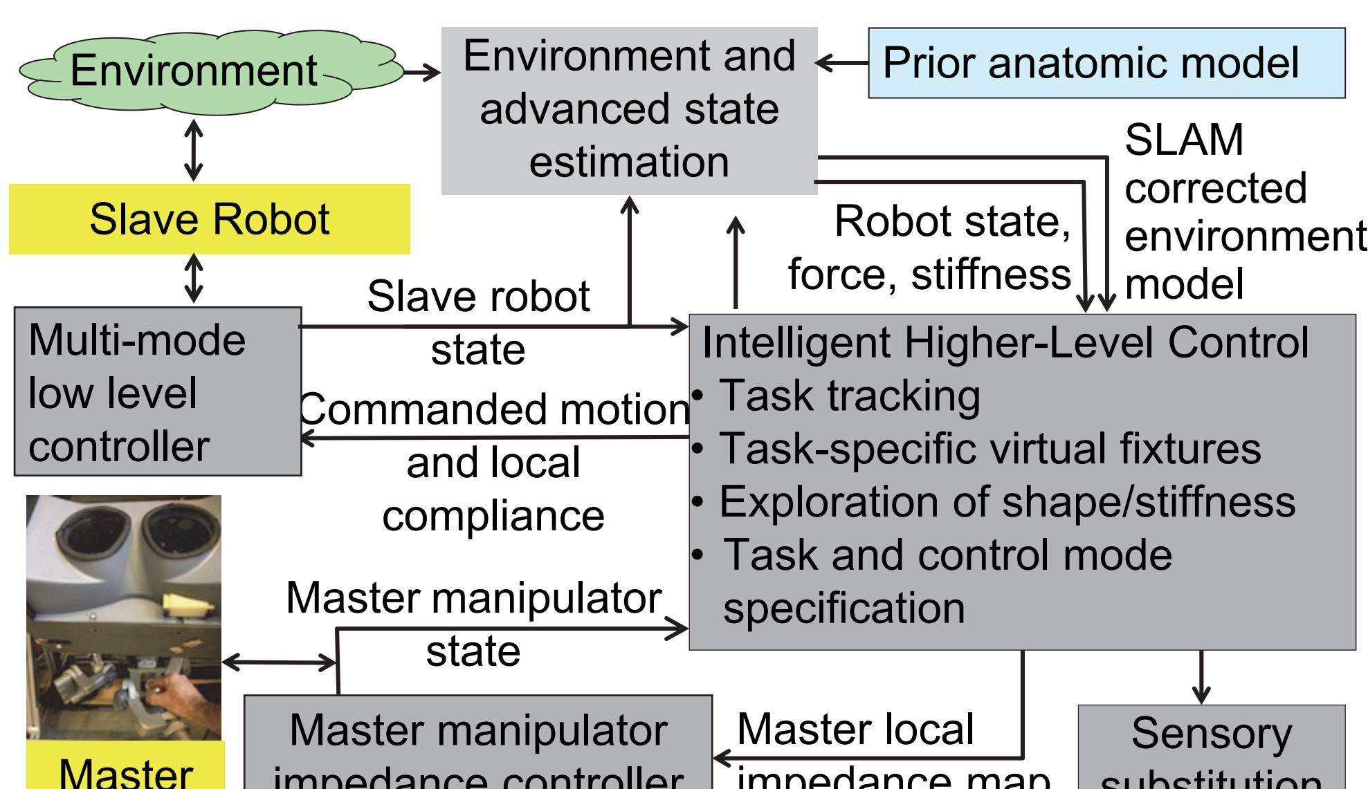
Telemansipation based on CSA includes the intelligent *high level controller* (HLC), the *low level controller* (LLC) of the master robot, LLC of the slave robot, and SLAM-based modeling block to correct the environment model.
