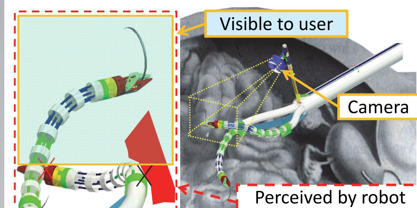
Intrinsic force sensing allows for the detection of contact in continuum robots. The robot can restrict movement to avoid collisions outside the surgeon's view.
