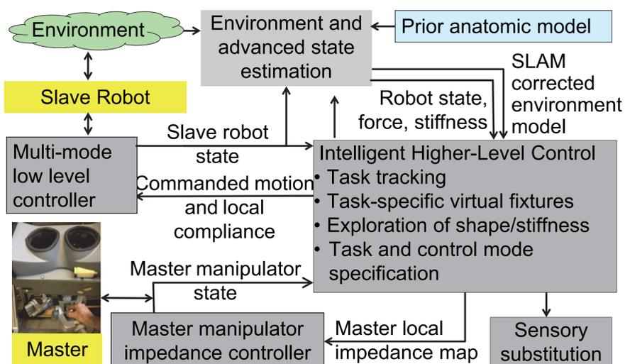
Telematipulation based on CSA includes the intelligent *high level controller* (HLC), the *low level controller* (LLC) of the master robot, LLC of the slave robot, and SLAM-based modeling block to correct the environment model.
