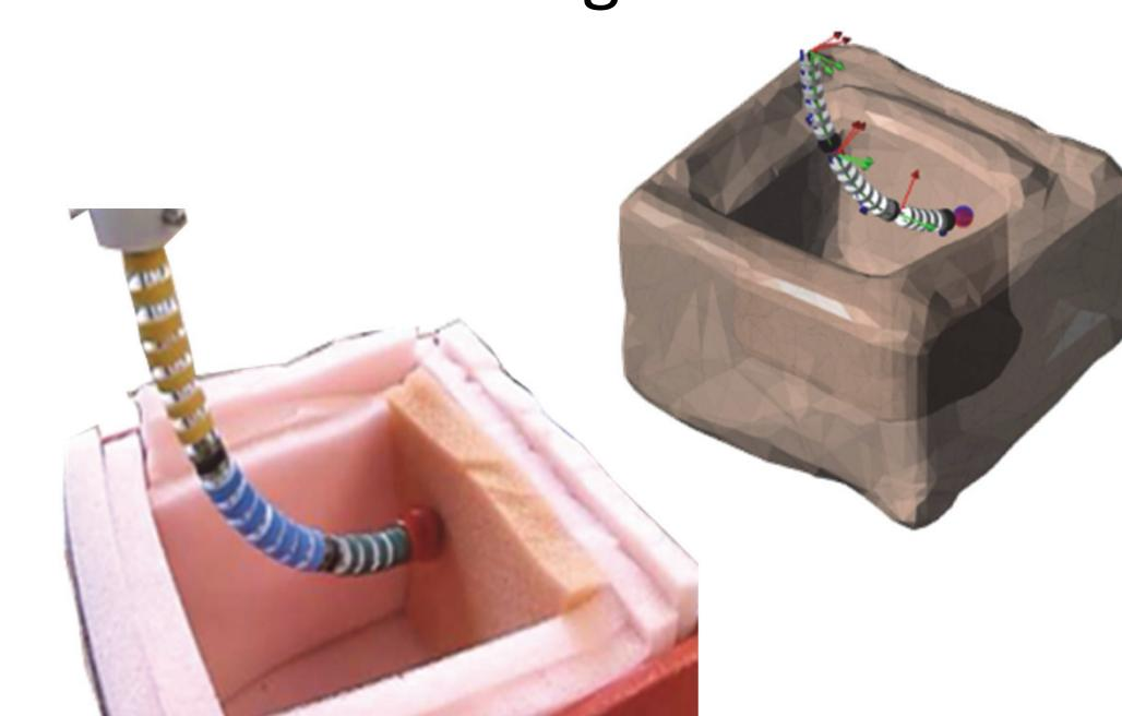
A combination of contact detection and constrained filtering has demonstrated the ability to register the robotic system to an unknown, flexible environment.
