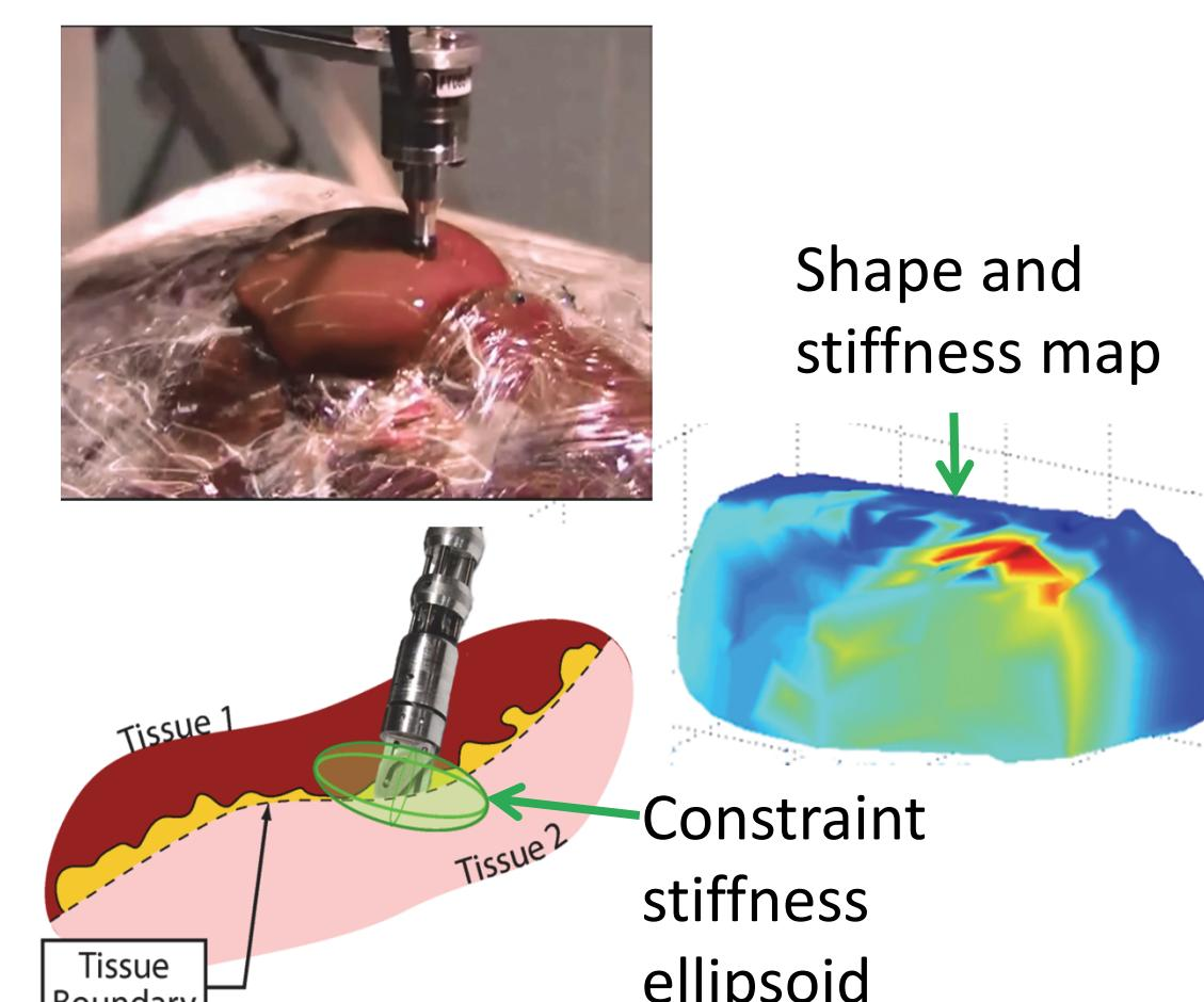
Stiffness information allows for constrained motion between tissue clefts.
