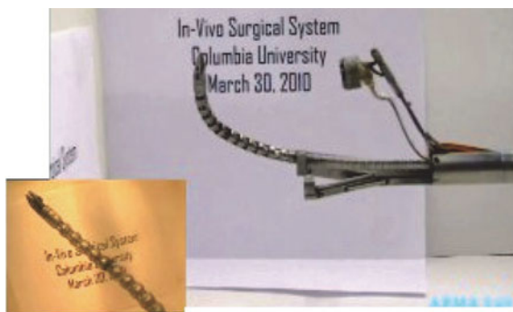
Fig. 20. One IREP arm with the camera mechanism deployed. The inset shows the view from the IREP camera.
