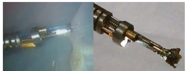
Fig. 10. Deployment of biopsy forceps. (Left) Laparoscope view of the system grasping bladder urothelium with a biopsy forceps and delivering parallel laser energy. (Right) Clinical view of a sample removed with combined grasping and laser delivery.
