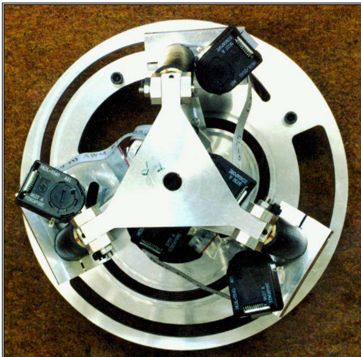
Figure 11.2: Top view of the RSPR prototype robot showing weight reduction voids in the base platform.
