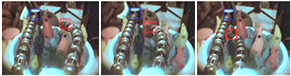
Fig. 5 Visual tracking of the IREP's dexterous arms
