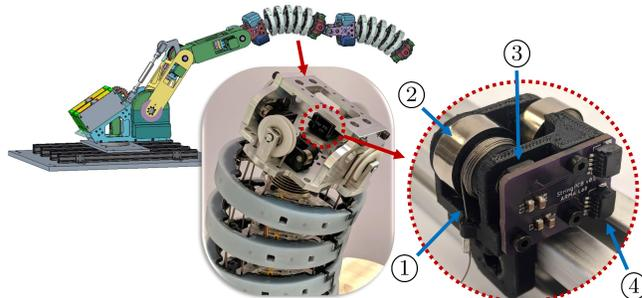
Fig. 1: In-situ collaborative robot with revolute joints and continuum segments. Each string sensor consists of ① a string, ② a constant torque spring, ③ a magnetic encoder, and ④ I<sup>2</sup>C bus connectors.
