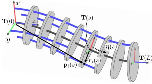
Fig. 2: Variables in our continuum segment kinematic model.
